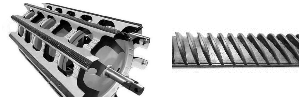
Figure 4. General view of the threshing drum and beater made of metal polymer
